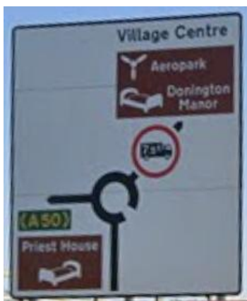
Figure 9. Advance direction sign (ADS) on approach to roundabout
